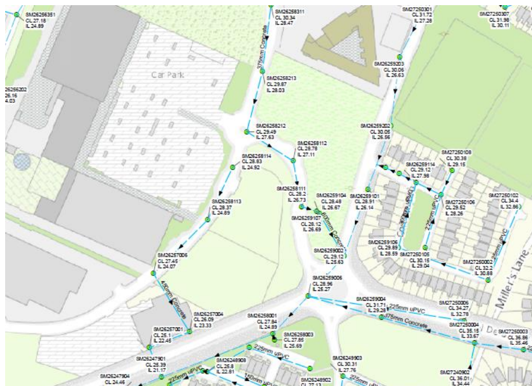
Figure 4.2 – Extract of Irish Water Surface Sewer Records.
